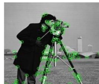
Fig. 10: Key point Localization in SURF[14]
